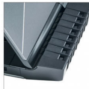
The display hinge has been set forward to make way for cooling components in the rear.
