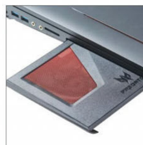
The Predator FrostCore module can replace the ODD drive for additional cooling.
